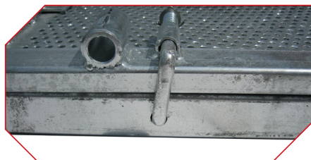
Locked stage barrier
